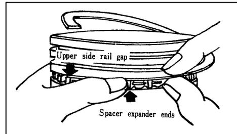
Install the lower side rail with its gap approximately 45 Degree right of the expander ends.
