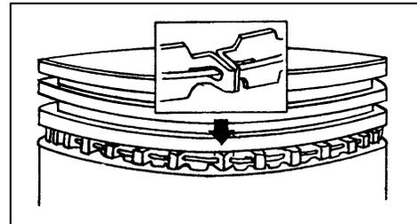
Hold with thumb the spacer expander with its ends completely butting. Install the upper side rail with its gap approximately 45 Degree left of Spacer Expander end.
